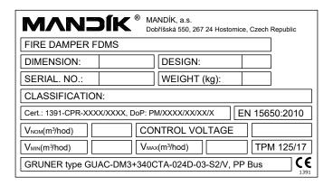
Data label FDMS with pressure control GUAC-PM3(-MB) - is placed on the damper casing (example)
