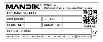
Data label FDMS with air flow control GUAC-DM3(-MB) - is placed on the damper casing (example)
