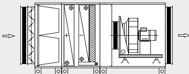
6) Unit for inlet of the air with blending, filtration system, water heating system and cooling
