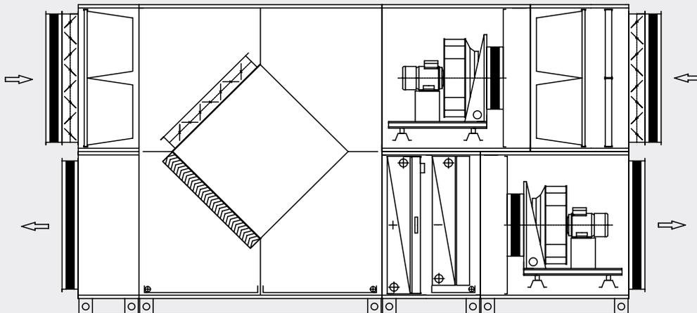
13) Unit for inlet and outlet of the air with rotational recuperator, mixing system, water heating system, cooling system and the fans with free impeller as well as the air buffers
