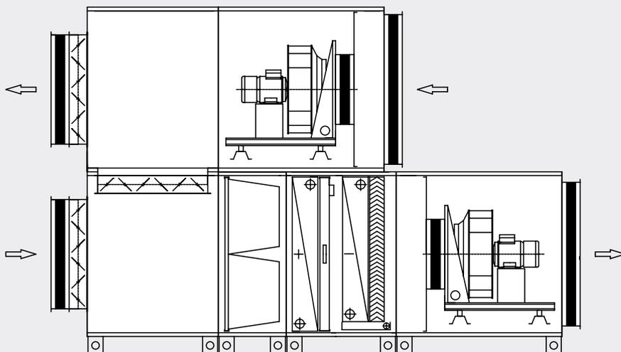
10) Unit for inlet and outlet of the air with plate heat exchanger, water heating system, and the fan with free impeller
