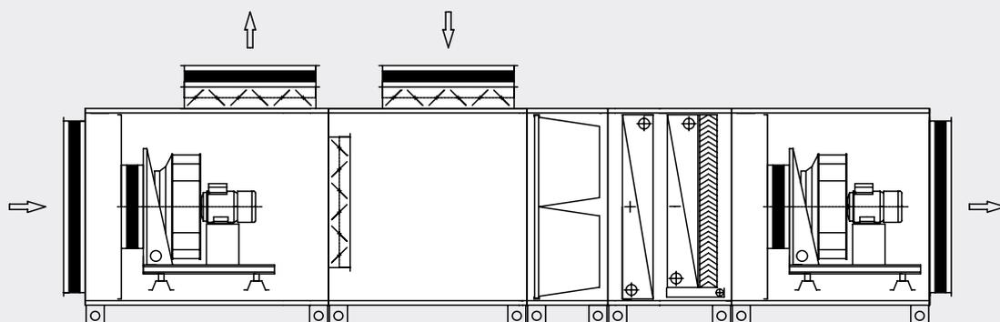
8) Unit for both inlet and outlet of the air with filtration system, water heating system, antifreeze protection, blending (one above another) and fans with free impeller
