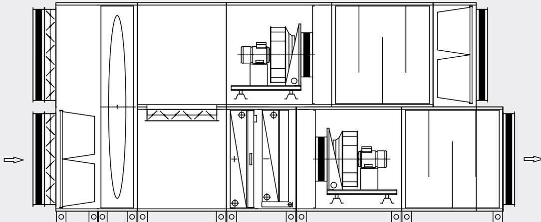
14) Outside unit for inlet of the air fitted with pre-heater, cooler and post-heater, fan with free impeller and chamber for steam moistener
