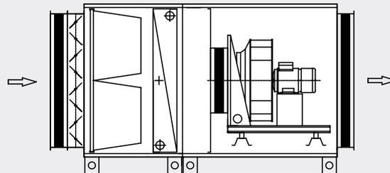
4) Unit for inlet of the air with filtration system, water heating system, fan with free impeller and noise buffer on discharge
