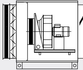
2) Unit for inlet or outlet of the air with filtration system and the fan with free impeller
