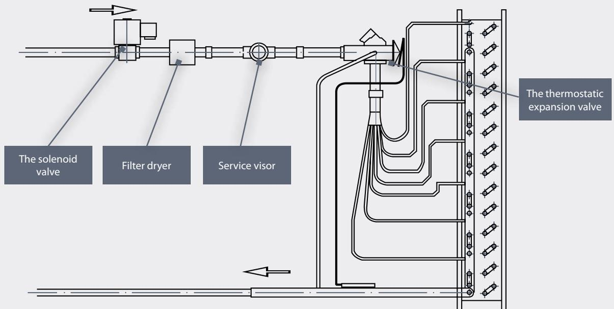
Fig. 4.10.1: Components of fluid section related to the cooling circuit before the evaporator.
