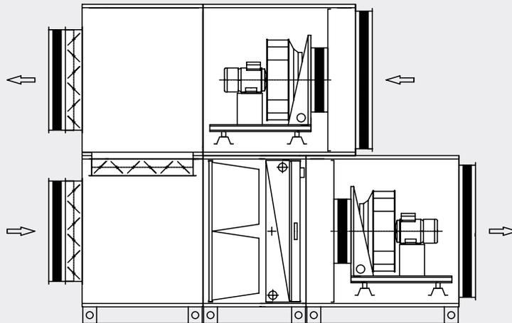
9) Unit for both inlet and outlet of the air with filtration system, water heating system, cooling system and blending (one above another)
