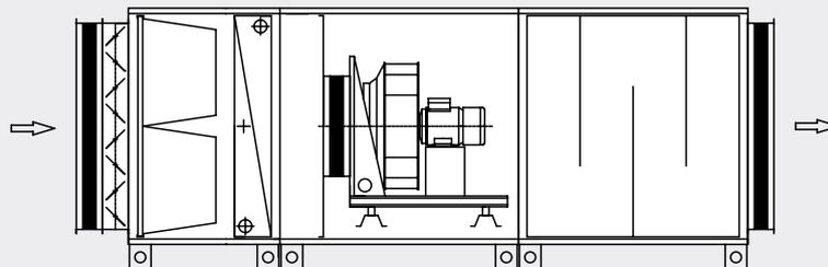
5) Unit for inlet or outlet of the air with filtration system, water heating system, cooling system and the fan with free impeller
