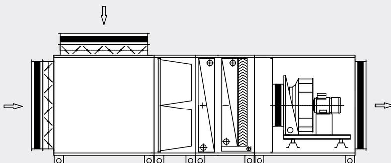
7) Unit for both inlet and outlet of the air with filtration system, water heating system, cooling system, blending (consecutive) and fans with free impellers
