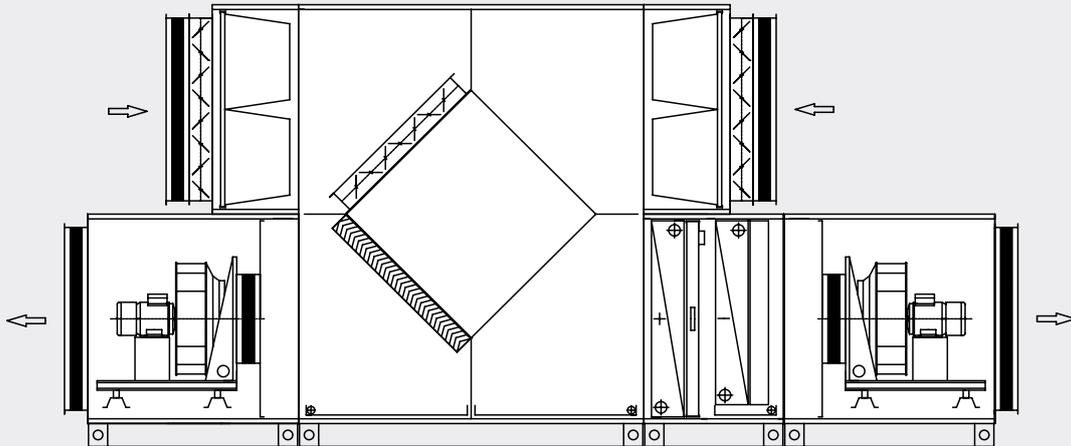
12) Unit for inlet and outlet of the air with plate heat exchanger, fat filter at the outlet, water heating system, cooling system and the fans with free impeller
