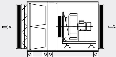
3) Unit for inlet of the air with filtration system, water heating system and the fan with free impeller
