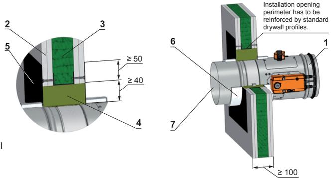
Installation in a gypsum wall construction
