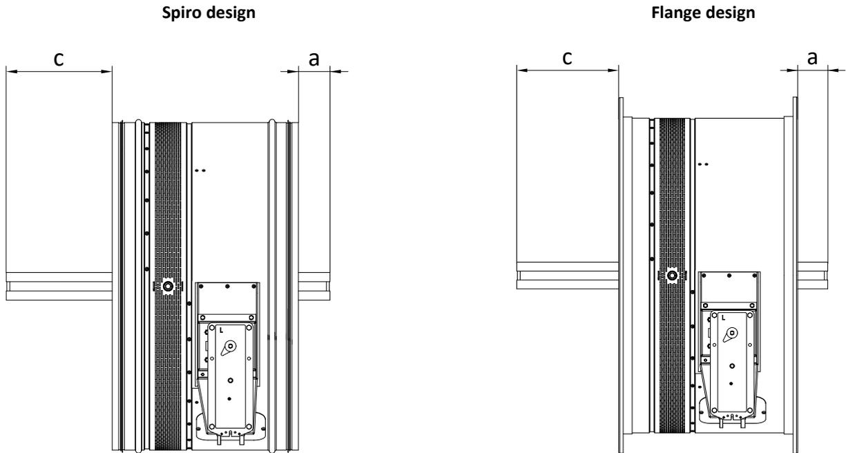
Values "a" and "c" has to be respected when projecting following air-conditioning duct.
