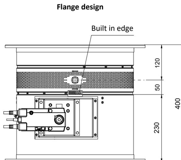
Dimensions of an installation opening
