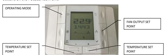
1) ROOM UNIT UPDATE - When power is connected and the connection is made to the controller, the room unit updates its data for a few seconds with the Climatix controller and the "P—" symbol is shown on the display.
