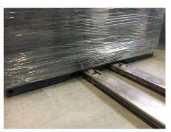
Openings are provided in the frame of the units for handling. During use, pallet truck forks must remain fully under the chamber.
