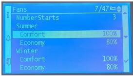
Press enter on the Comfort supply / return fan row and use the arrows to adjust the fan output value [%] – use the arrows to change the value and the press enter to confirm.
