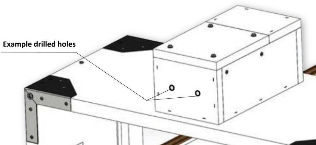
*Example of position of holes in the wall of the box, without pre-manufactured slot*
