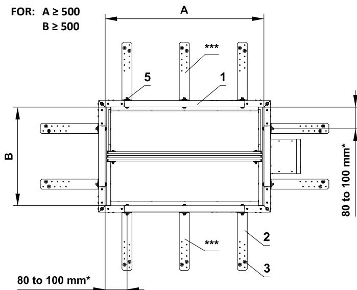
Fixing element/steel holder for connecting damper to the wall (optional accessories MANDIK, a.s.)
