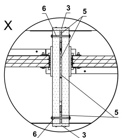
**2 dampers on top of each other - solid wall - Ablative Coated Batt system****EI 120 S**
