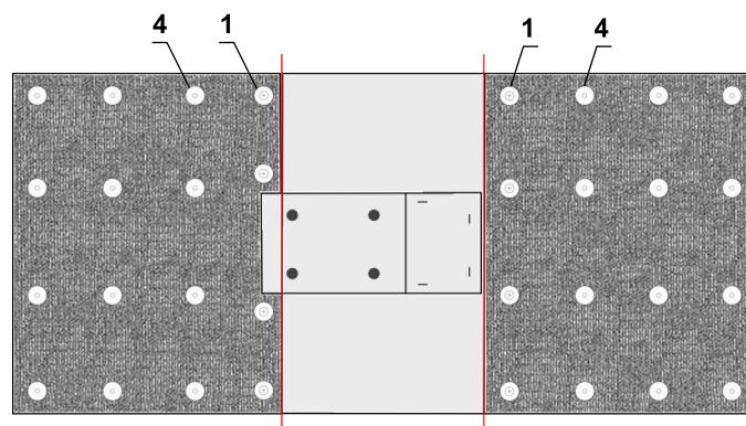
Insulation cut-out area around the actuator cover
