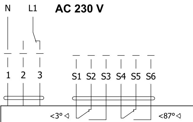
Extended leads are not possible with smoke control dampers as the belimo cables are not fire rated to a high Field wiring must be brought into and terminated within the damper housing. For more detail → see pages 55 to 57, paragraph Assembly.
