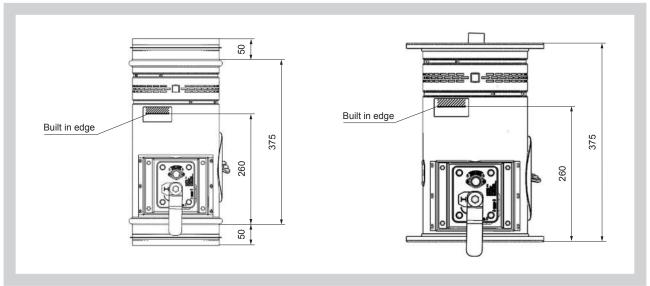
For dampers with installation holders is valid maximal built in edge
