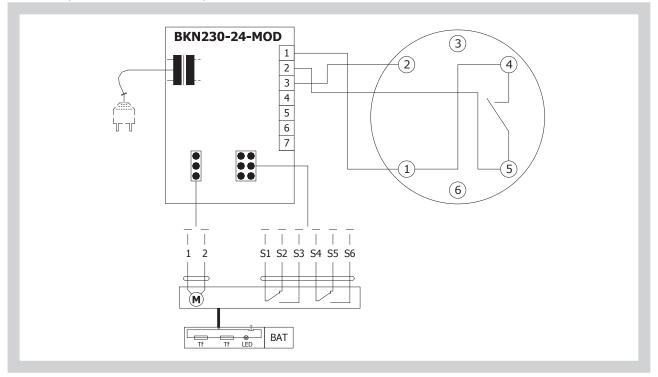
Design with the communication and supply device BKN 230-24MP and actuating mechanism BF 24TL-TN-ST for connection to MP-Bus. BKN 230-24MP supplies to intelligent actuating mechanisms of fire dampers BF 24TL-TN-ST decentrally needed power supply. In this way can be realize long MP-Bus communications (up to 800 m). Up to 8 Bus nodes can be parallel connected and controlled by Master device (DDC with interface). More information in Belimo catalogue.
