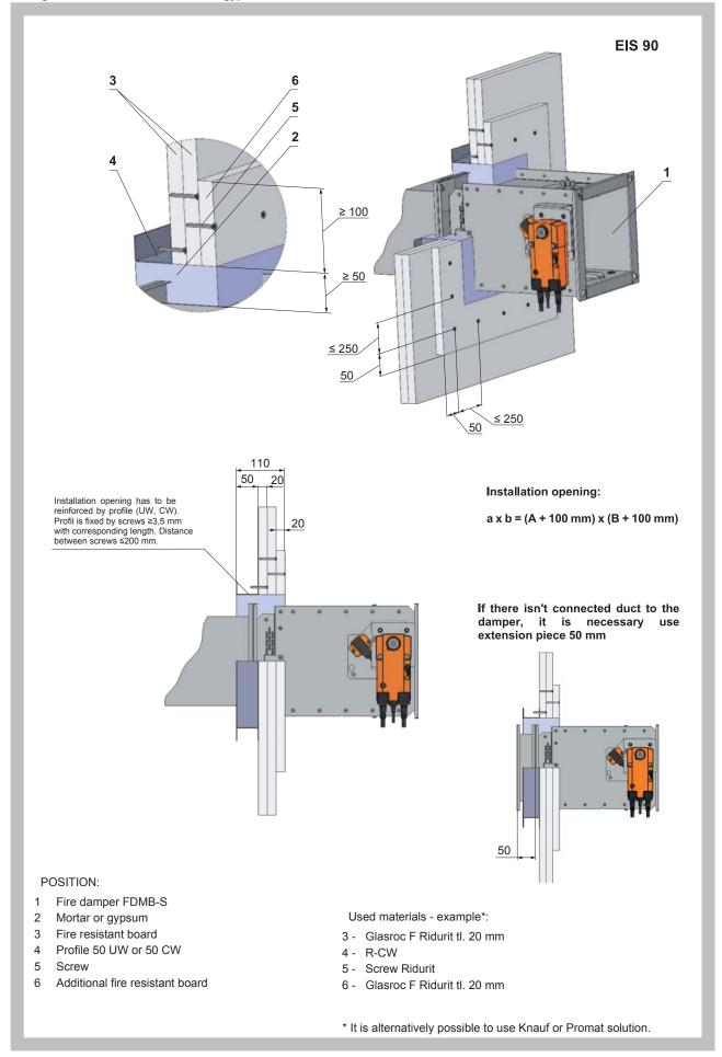
Fig. 94 Thin shaft wall - Installation frame E1 - RECTANGULAR DAMPER
