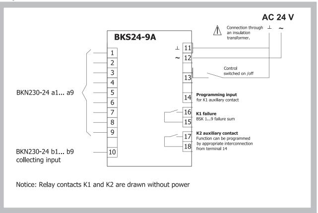
Tab. 3.2.2. Communication and control device BKS 24-9A
