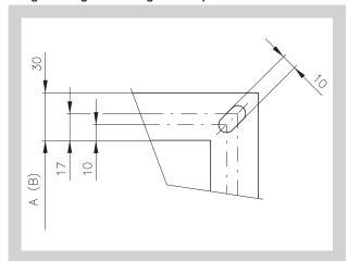
Fig. 35 Flage of rectangular damper - INSTALLATIONS SIDE
