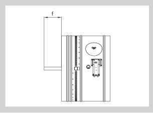
Fig. 33d Damper for SPIRO duct
