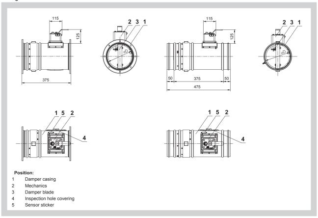
FDMB with actuating mechanism - round Fig. 32
