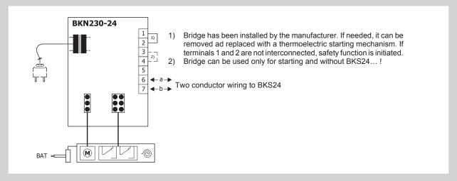
Design .61 with communication and supply device can be complemented with smoke detector ORS 142 K. For supply and comunnication is used BKN 230-24-C-MP, which together with the BF 24TN-ST (BFL 24T-ST, BFN 24T-ST) enables central control and checks of fire damper by means of a simple 2-conductor wiring and it also allows connection to the system via MP-BUS communication. More information in the Belimo catalog.
