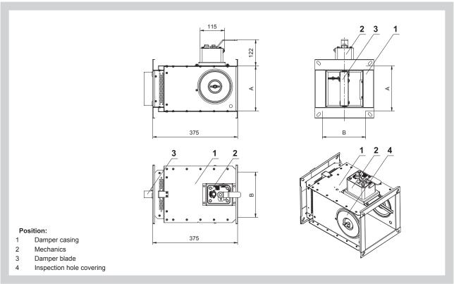
Fig. 30 FDMB with actuating mechanism - rectangular
