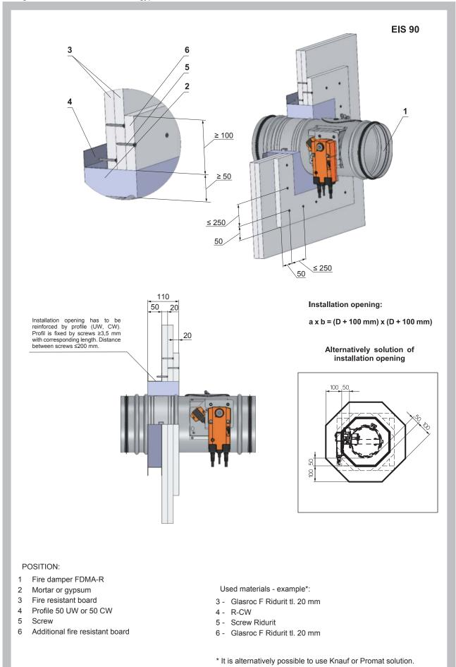
Fig. 96 Thin shaft wall - Installation frame R1 - ROUND DAMPER
