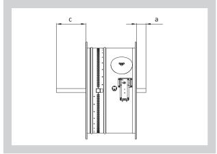
Fig. 33c Blade overlaps - round damper SPIRO
