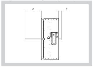
Fig. 33b Blade overlaps - round damper
